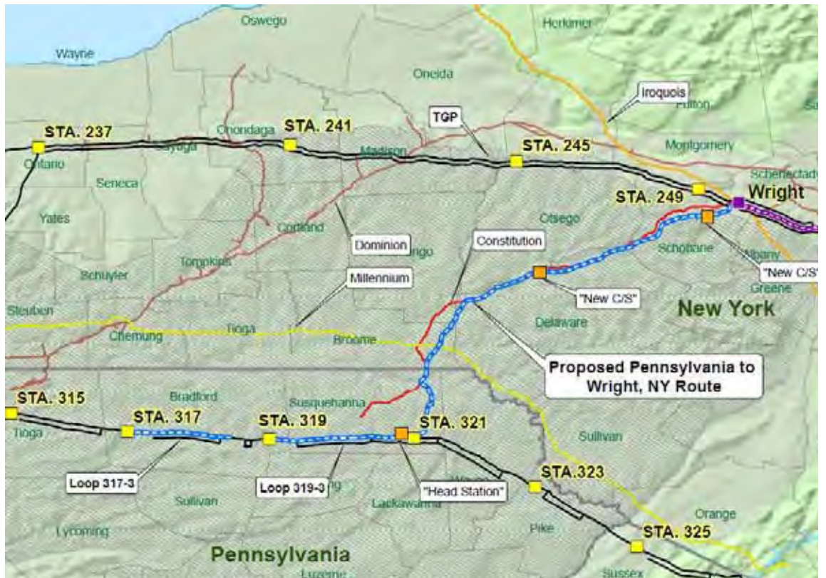
Map of a distribution system for natural gas showing regional pipelines, including the proposed Northeast Energy Direct or "Proposed Pennsylvania to Wright, NY Route" (broad dashed gray line) and "Constitution" (narrow solid black line). Where the two would be co-located, only gray line of NED is shown. Compressor stations are shown along the pipelines, including existing (light gray squares, labeled "STA. #") and proposed (medium gray squares labeled "New C/S" or "Head Station"). A color version is available on line @ franklinlocal.org/nfr .
