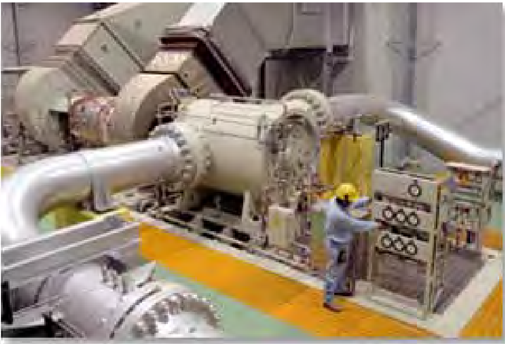
Solar Turbine model Titan 130 turbine and C65 compressor producing 20,500 hp to move 20,000 cu ft per min at 1,600 psi. The compressor is the cylinder in the center with 30 inch input and output gas pipelines. The turbine is the smaller cylinder upper right, between the air intake and exhaust. Photo: Solar Turbines, Inc.
