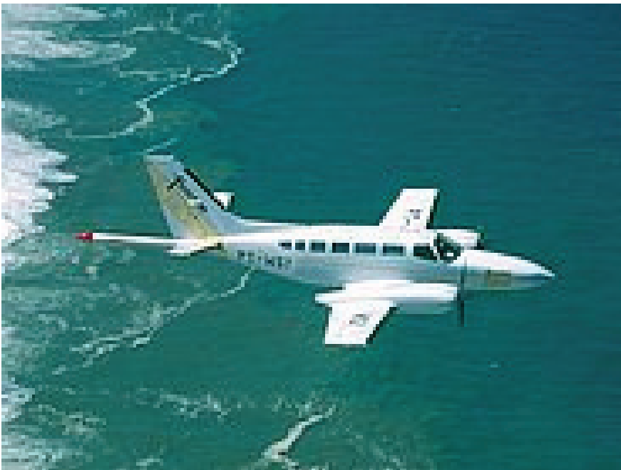
Cessna 404 outfitted with a Magnetic Anomaly Detector
